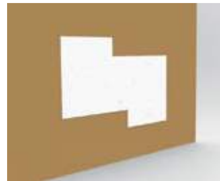
2. Use the provided template to drill the holes and paint the drywall.
