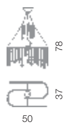
Silk Alpha lampadario 50 cm L 50 cm - H 78 cm - SP 37 cm 4 x G9 40W
