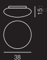
Bianca PL 38 1x100W E27 inc. 1x20W PLE-T EL 1x42W G24q3 FL 1x26W G24d3
